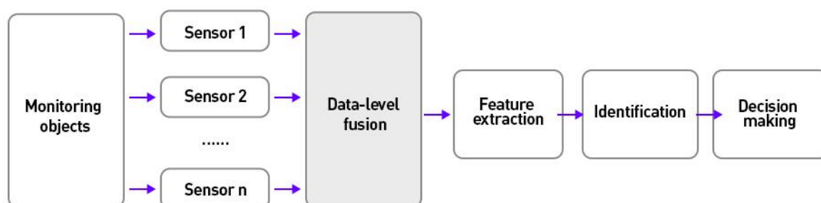
Schematic diagram of the basic principles of multi-sensor front fusion
